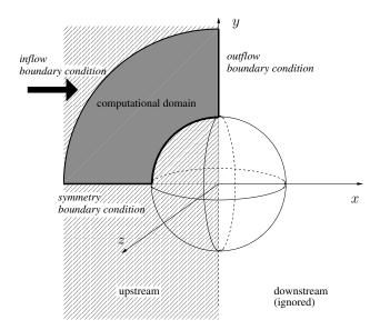
Figure 10: Axisymmetric flow around a sphere: geometry and computational domain. By rotational symmetry and by symmetry with respect to the axis x, the computational domain is included in the plane (x, y, 0). The downstream flow is not simulated.
