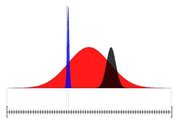
Figure 3: Three different distribution functions and a global grid that satisfies (7)-(8): the bounds are given by the largest distribution, the step is given by the narrowest distribution.
