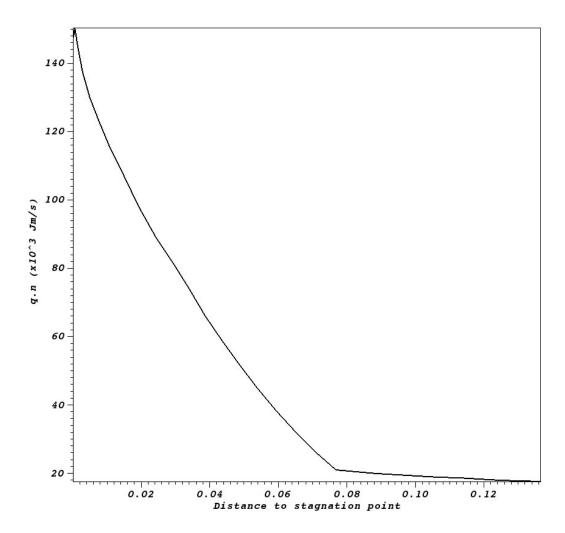
Figure 18: 3D flow around a cone: normal heat flux along the boundary (computed with the kinetic code and the AMR velocity grid).
