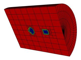
Figure 14: 2D axisymmetric flow around a sphere: cylindrical AMR velocity grid computed with Rankine-Hugoniot relations rather that with the CNS pre-simulation, with contours of the corresponding support function. Note that the refined zones are much smaller than in the previous grid, and that the contours of the support function are different (see figure 12)
