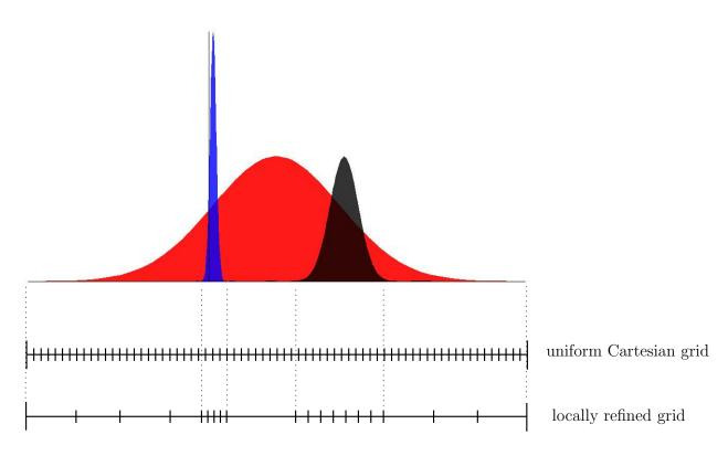
Figure 4: Three different distribution functions (top), the corresponding uniform Cartesian velocity grid (middle), and the grid locally refined in the support of the distributions (coarsened elsewhere).
