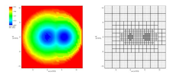
Figure 8: Plane flow around a cylinder. Left: support function, Right: velocity grids (solid line: induced AMR velocity grid, dotted line: initial fine Cartesian grid).
