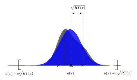
Figure 2: Support of a distribution function f(x, .): the distribution (in black), its corresponding Maxwellian (in blue), and the corresponding support based on the bulk velocity u and the temperature T.
