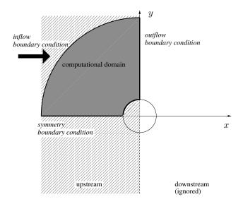
Figure 6: Plane flow around a cylinder: geometry and computational domain. By symmetry with respect to the axis x, the computational domain is defined for y>0 only. The downstream flow is not simulated.
