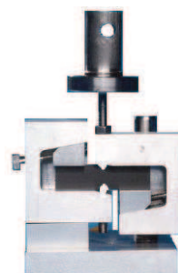
Fig.1. Iosipescu experimental device
