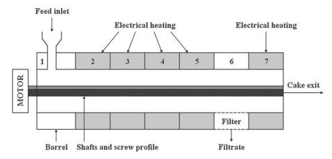
Fig. 1. Schematic modular barrel of the Clextral BC 21 twin-screw extruder used for extraction of oil from jatropha seeds.
