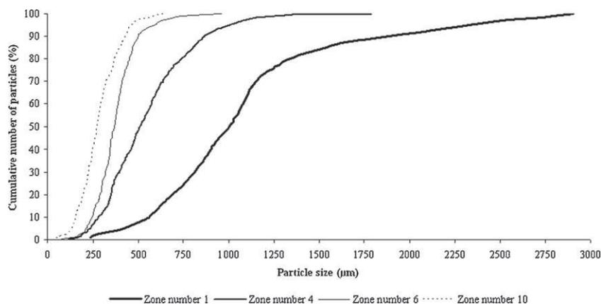
Fig. 4. Cumulative number of particles as a function of particle size for the matter inside, collected at the end of trial 13, in zones 1, 4, 6, and 10 along profile 4.
