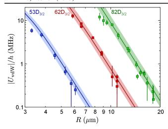
FIG. 3 (color online). Magnitude  $|U_{\rm vdW}|$  of the interaction energy between atoms in  $|nD_{3/2}, m_j = 3/2\rangle$ , extracted from the fits of Fig. 2, versus R, for n = 53 (blue), n = 62 (red), and n = 82 (green). Error bars are one standard deviation in the fitted  $|U_{\rm vdW}|$ . Solid lines: *ab initio* theoretical expectations (see text) without any adjustable parameter. Shaded areas: 5% systematic uncertainty in R.
