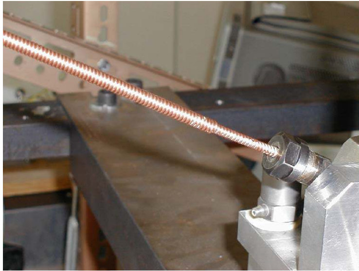
Fig. 2. Test specimen: steel wire surrounded by copper wire.
