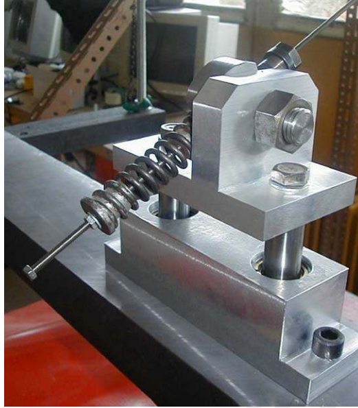
Fig. 3. Sub system assembly with the stressing anchorage.
