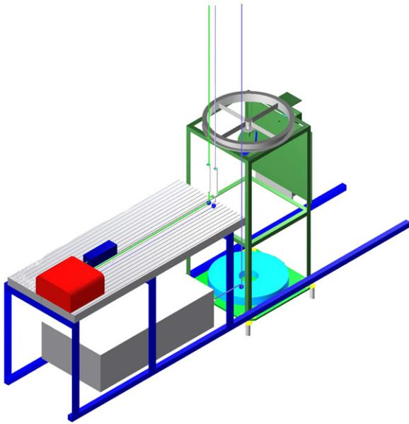
Fig. 1. The LOANA instrument setup within the lidar at DDU. The blue unit is the Nd:YAG laser, the red unit hosts the harmonic generators, and the gray unit at the bottom is the excimer laser.
