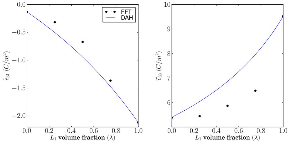
Figure 2: Overall piezoelectric coefficients  $\tilde{e}_{31}$  and  $\tilde{e}_{33}$  for 2-1-2 epoxy/PZT composite as a function of the piezoelectric layer volume fraction ( $\lambda$ ). FFT computations have been performed for  $\lambda = 0, 0.25, 0.5$  and  $0.75$ .
