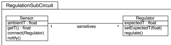
Fig. 15 Regulation Circuit Submodel
