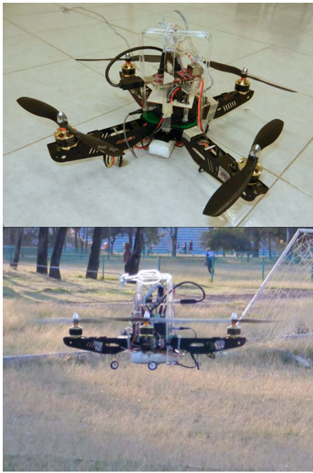
Fig. 3. The quadrotor mini-helicopter in flight
