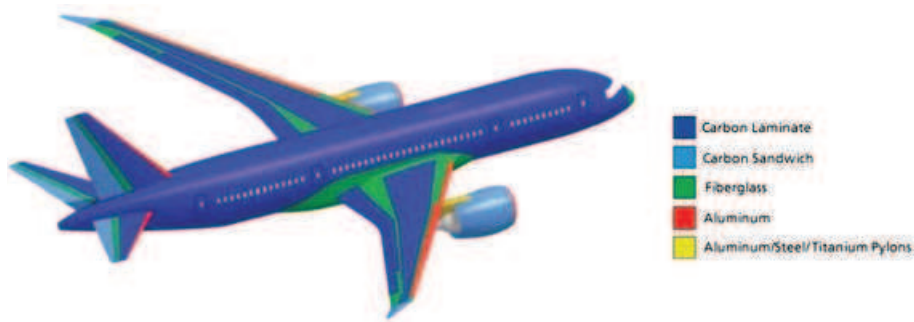
Figure 1. Boeing 787 material distribution [25].
