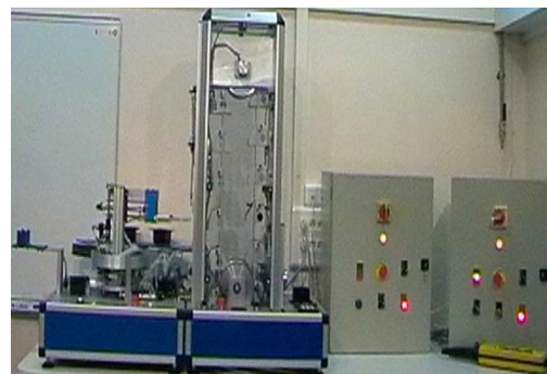
Fig. 6. Vertical store system.
