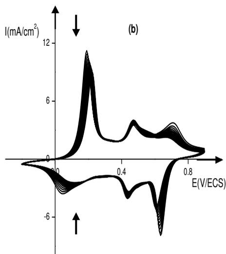
**Figure 1:** Cyclic voltammograms relating to polyaniline (PAn/Pt), in  $\text{H}_2\text{O}/[\text{LiClO}_4 (0.1 \text{ M}) + \text{H}_2\text{SO}_4 (0.5 \text{ M})]$  solution, obtained at  $v = 10 \text{ mV/s}$ , between  $-0,2$  et  $0,9 \text{ V/SCE}$ .
