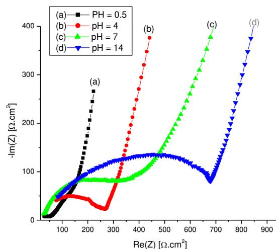
**Figure 2:** Nyquist diagrams related to the films of PAn/Pt, obtained for different values of the pH of the solution:  $\text{H}_2\text{O}/(\text{LiClO}_4 0.1\text{M} + \text{H}_2\text{SO}_4 0.5\text{M} + \text{An } 2.10^{-1}\text{M} + \text{NaOH } 1\text{M})$ , and analyzed in a solution without monomer.
