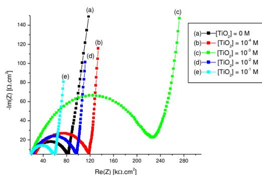
**Figure 3:** Nyquist diagrams relating to the  $(\text{PAn} + \text{TiO}_2)/\text{Pt}$  films in a solution free of monomer  $\text{H}_2\text{O}/(\text{LiClO}_4 \text{ 0.1M} + \text{H}_2\text{SO}_4 \text{ 0.5M})$ , recorded on a frequencies range between  $10^5$  Hz and  $10^{-1}$  Hz, at the open circuit potential, with a disturbance of 10 mV. The film is obtained from solutions containing different concentrations of titanium oxide.
