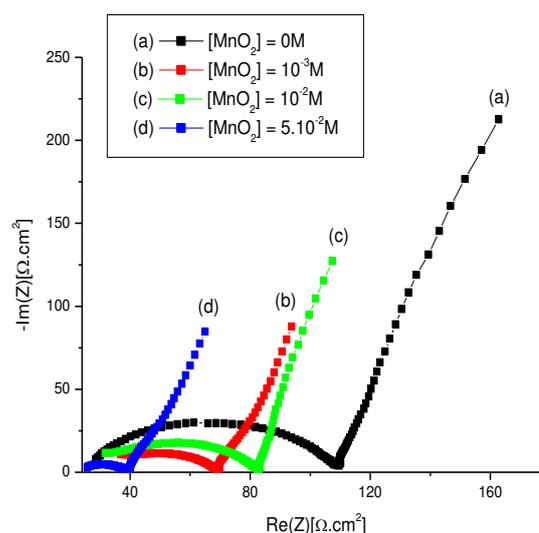
**Figure 4:** Nyquist diagrams related to the films of composite  $(\text{PAn} + \text{MnO}_2)/\text{Pt}$ , obtained for different concentrations of  $\text{MnO}_2$ , indicated on curves, analyzed in a solution containing no monomer and  $\text{MnO}_2$ .
