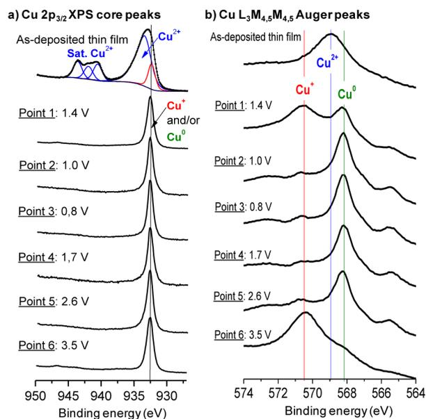
**Figure 3.** XPS analyses of (a) Cu  $2p_{3/2}$  XPS core peak and (b) Cu  $L_3M_{4,5}M_{4,5}$  Auger peak performed onto cycled CuO thin film electrodes at different stages of the first cycle: the as-deposited thin film, upon discharge (points 1, 2, and 3) and during the charge (points 4, 5, and 6).
