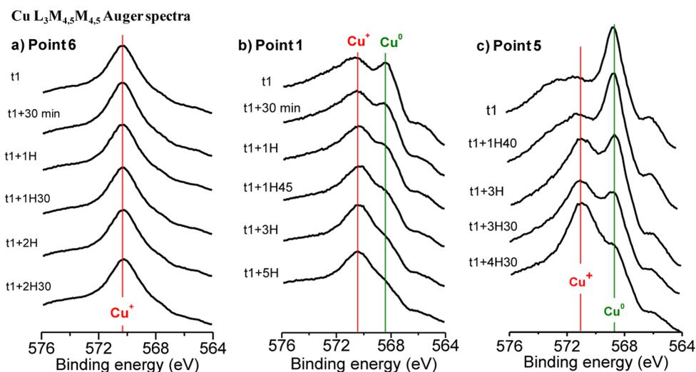
**Figure 7.** Depth analysis performed onto cycled CuO thin film electrodes: the Cu  $L_{3}M_{4.5}M_{4.5}$  Auger peak was recorded at different times of an argon ion etching, and results are given for point 6 (a), point 1 (b), and point 5 (c).
