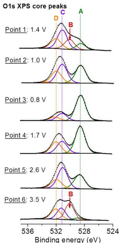
**Figure 4.** XPS analyses of the O 1s core peak performed onto lithiated CuO thin film electrodes at different stages of the first cycle: upon discharge (points 1, 2, and 3) and during the charge (points 4, 5, and 6).
