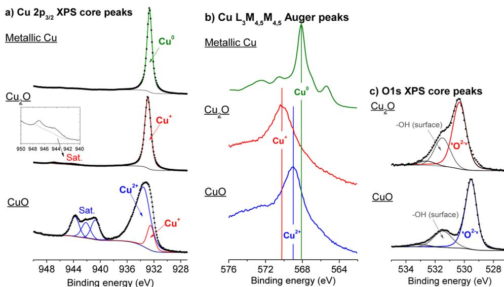
**Figure 1.** XPS spectra (Cu  $2p_{3/2}$  and O  $1s$  core peaks) and Auger spectra (Cu  $L_3M_{4,5}M_{4,5}$  peak) of the Cu,  $Cu_2O$ , and CuO references.  $Cu_2O$  and CuO samples are thin films elaborated by RF magnetron sputtering, while the Cu sample is a foil etched before the XPS analysis to fully remove the surface oxide layer.
