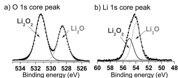
**Figure 6.** O 1s (a) and Li 1s (b) XPS core peak spectra of a commercial powder containing a mixture of Li<sub>2</sub>O<sub>2</sub> and Li<sub>2</sub>O compounds.
