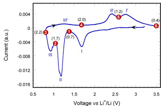
**Figure 2.** Voltammogram of the first cycle of a Li/CuO cell performed between 0.8 and 3.5 V at a scan rate of 5.0  $\mu\text{V s}^{-1}$ . The dots indicate the samples studied by XPS at different stages of the first cycle, with their corresponding Li<sub>x</sub>CuO overall composition (*x* values) between brackets.
