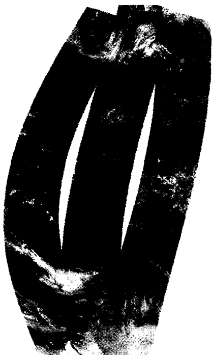
Fig.1. Image constructed from 670 nm reflectance measured by POLDER on 10 November 1996 along three ADEOS paths (orbit numbers 3107 to 3109) over the Atlantic Ocean. Clouds appear as light shades against a darker ocean or land background.
