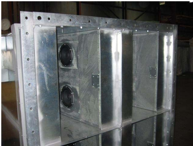
Image 13: Active Noise Attenuator Showing Speakers
