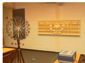
Figure 7: Acoustic Camera set-up and acoustic wall panels
