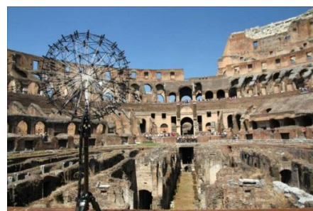
Figure 12: Acoustic Camera set-up in Rome Coliseum.
