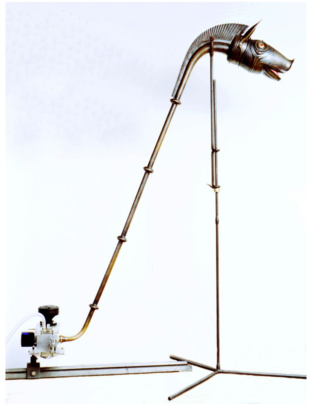
Figure 1: The Deskford carnyx reconstruction, sounded by an artificial mouth in the Musical Acoustics Laboratory at the University of Edinburgh.
