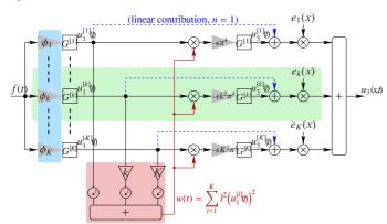
Figure 3: Block-diagram of an  $o(\epsilon)$ -simulation of Eq. (1) with K modes: the dashed arrows isolate the linear dynamics (n=1) of each mode; the shaded central part isolates the  $o(\epsilon)$ -dynamics of a mode k; the shaded bottom part isolates the dynamics of the integral term in (M1) (gains 1, k and K before the square operators are due to  $\partial_x$ ); the shaded left part corresponds to simple gains, controlled by the spatial distribution of the excitation force.
