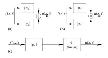
Figure 5: Sum (a), product (b), and cascade (c) of two Green-Volterra systems f.
