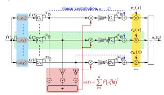
Figure 8: Block-diagram of an  $o(\epsilon)$ -simulation of Eq. (1) based on Green-Volterra kernels with *K* modes: the excitation force f(x, t) is completely unknown to the system and is decomposed on the modal basis using a scalar product.
