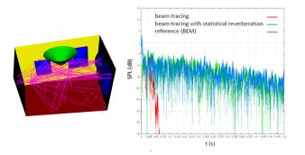
Figure 3: Example of beam-tracing: paths (left), impulse response (right, with and without statistical reverberation).
