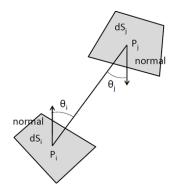
Figure 5: Form factor for radiosity.
