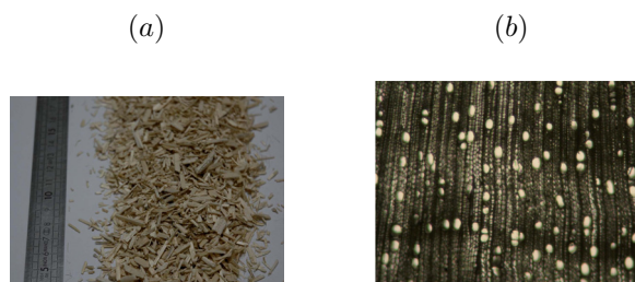
Figure 1: Photographs showing mix of hemp particles S_A ((a) shows the characteristic dimension of the particles and (b) shows the intraparticle porosity)
