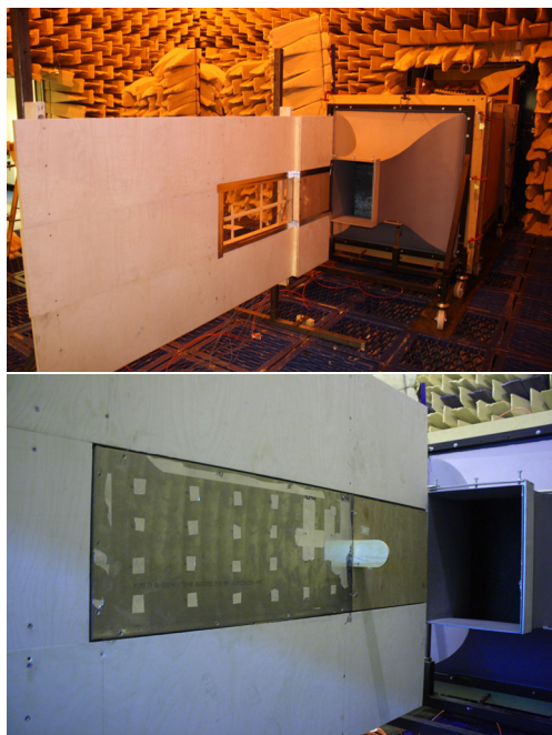
Figure 1: General view of the experiment set-up for the step case and the wing mirror case.
