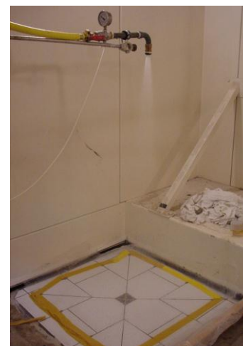
Figure 3: Measurement setup for evaluating the water jet noise level (source: reference water jet (INS) at 2 m oriented to the center of the shower area).
