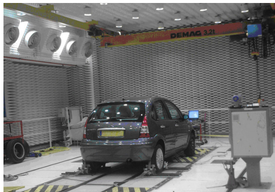
Figure 11: Roller bench used for transfer function measurement
