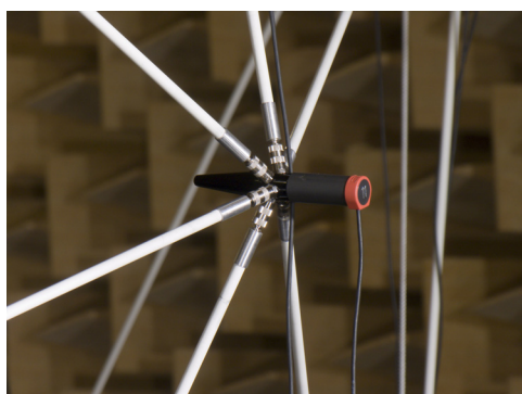
Figure 3: Close-up of the microphone array without additional absorbers, electret capsule at the narrow end of the conical shape, preamplifier in the rear end
