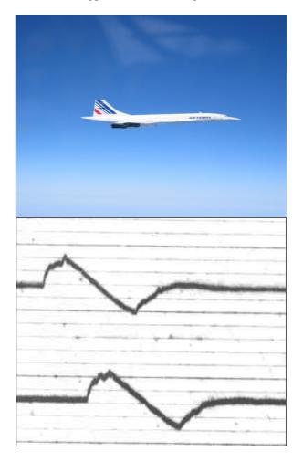
Figure 5 : Sonic booms of Concorde at 30 km
