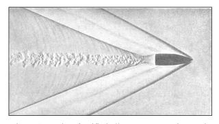
Figure 1 : Wake of a rifle bullet at a supersonic speed
