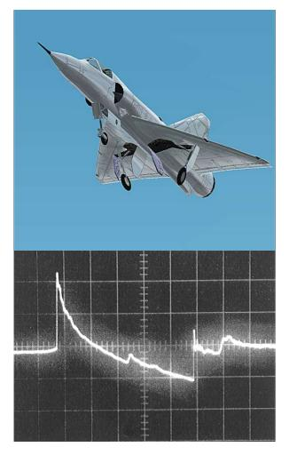
Figure 4 : Sonic boom of a Mirage III in acceleration
