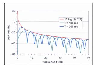
Figure 3 : N-wave spectra and tangent curve
