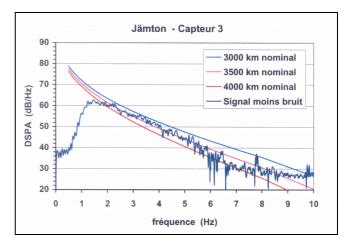
Figure 21 : Estimation of the distance of Concorde
