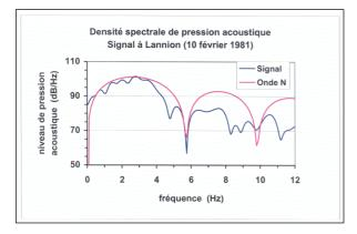
Figure 8 : Real and theoretical spectra of sonic boom
