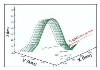
Figure 6 : Sound ray tracing in approach of Brittany
