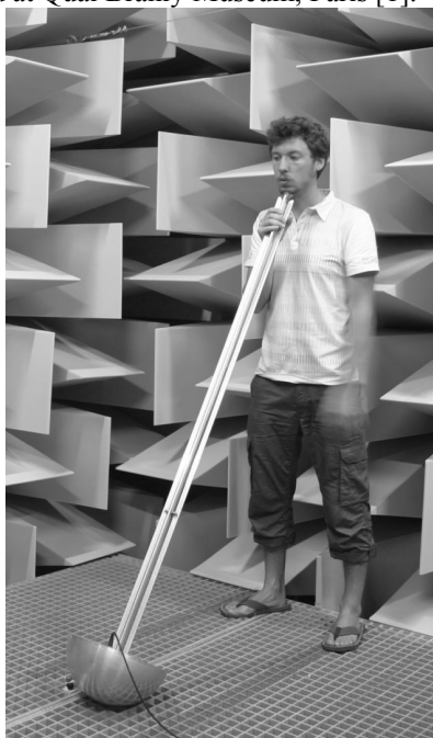
Figure 1: User with bone conduction device in anechoic room at LAUM
