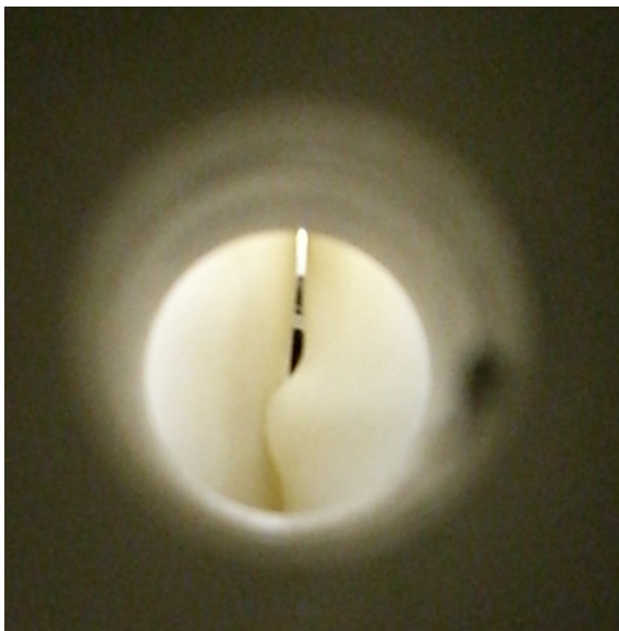
Figure 9: Picture of the glottal replica. Vocal fold with artificial growth is on the right side.
