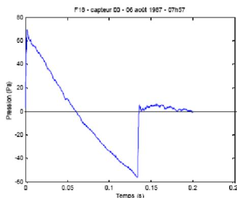
Figure 2: N-wave under track
