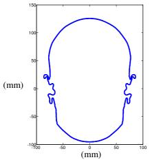
Figure 1: Contour generated by the *P* points in slice 1 of the KEMAR model.
