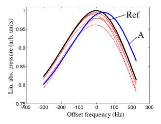
Figure 14: Ref - original HRTF. Putty at A shifts peak more than putty at U to Z (dashed lines).
