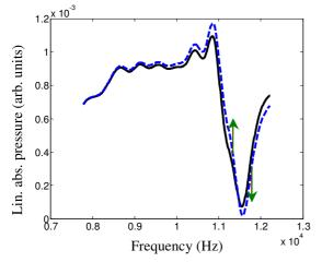
Figure 7: Line - original HRTF with notch. Dashes - HRTF plus weighted sum of  $\Delta$ HRTF s. Arrows indicate morph vector values.
