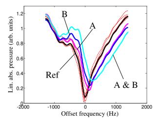
Figure 12: Ref - original HRTF. Putty in active regions A & B shifts notch more than putty at U to Z (dashed lines).
