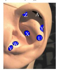
Figure 13: Putty sites used to validate peak analysis.
