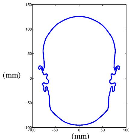
Figure 1: Contour generated by the  $P$  points in slice 1 of the KEMAR model.
