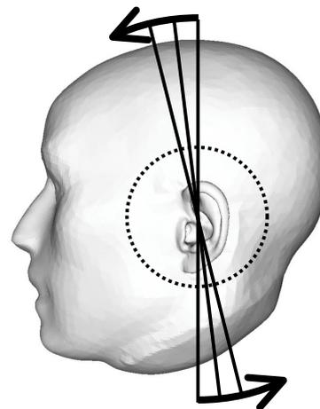
Figure 2: Template head radial slicing. Dotted line - an idealised cross-slice contour.
