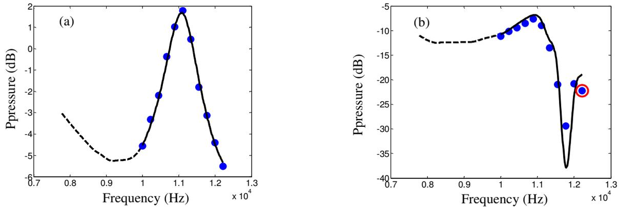
Figure 6: (a) HRTF for 1 m above the head. Line: HRTF for reference mesh; dots: HRTF for MPA-FD mesh. (b) HRTF for 1 m behind the head. The ringed point fails the similarity test
