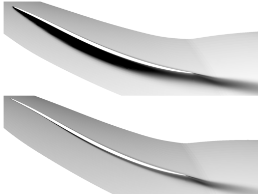
Figure 5: Influence of angle \alpha on the turbulence kinetic energy.
