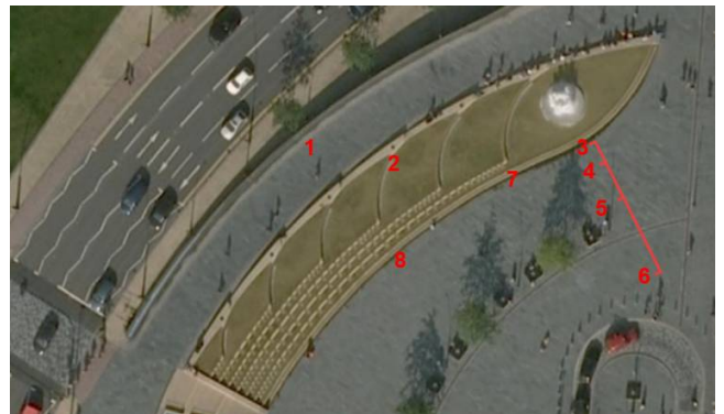
Figure 11: Plan of the Sheaf Square [based on googlemap], showing a range of water features, and the measurement points: 1, Steel barrier; 2, Medium cascade; 3-6, Big fountain (1,3,5,10m); 7, Small cascade L1; 8, Small cascade L3.
