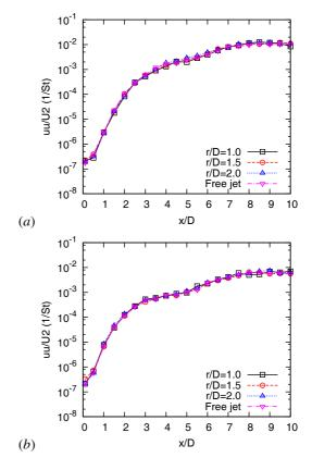
Figure 3: Evolution of velocity fluctuations on the jet centerline for M = 0.4 and St = 0.4 (*a*) and St = 0.6 (*a*).
