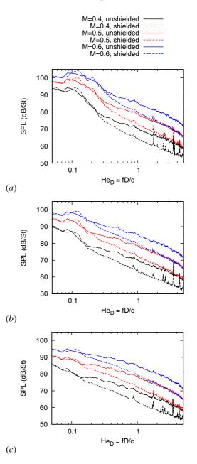
Figure 5: Sound spectra as a function of Helmholtz number measured by the shielded and unshielded microphones for r/D = 1 (*a*), r/D = 1.5 (*b*) and r/D = 2 (*c*)
