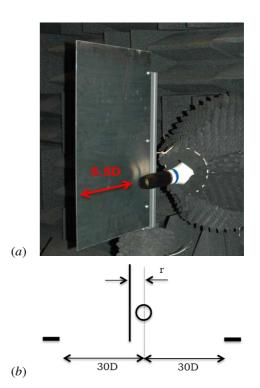
Figure 1: (*a*) Jet-wing setup; (*b*) Schema showing microphone positions
