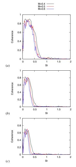
Figure 7: Coherence between the two diametrically-opposed microphones for r/D = 1 (*a*), r/D = 1.5 (*b*) & r/D = 2 (*c*).
