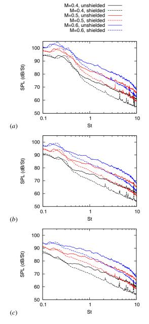
Figure 4: Sound spectra as a function of Strouhal number measured by the shielded and unshielded microphones for r/D = 1 (*a*), r/D = 1.5 (*b*) and r/D = 2 (*c*)
