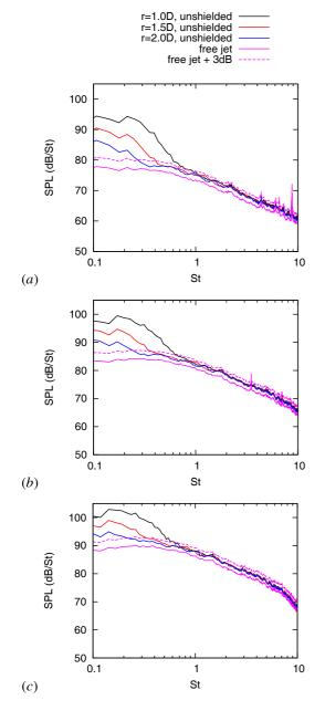
Figure 6: Effect of distance between the plate and the jet centerline on sound radiation for the M = 0.4 (*a*), M = 0.5 (*b*) and M = 0.6 (*c*) jets
