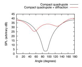
Figure 9: Sound radiation by a compact quadrupole at free space and in the presence of a semi-infinite flat plate.
