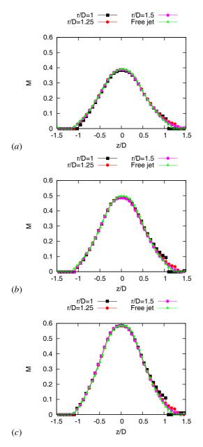
Figure 2: Mean velocity profiles at x/D = 5.6 for the M = 0.4 (*a*), M = 0.5 (*b*) and M = 0.6 (*c*) jets
