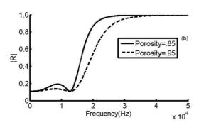
Figure 1: Effect of porosity on frequency dependence of a plane sound wave incident at  $60^{\circ}$  on a 6mm APPM layer of  $BaTiO_3$ .
