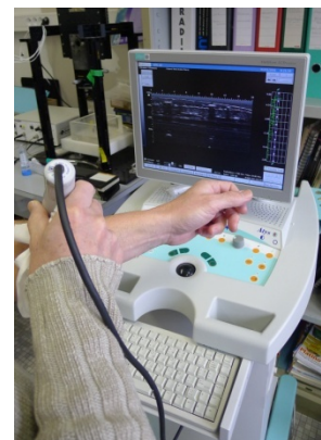
Figure 7: Photograph of the high frequency (20 – 50 MHz) ultrasound imaging system [17] (for in vivo human forearm skin images).
