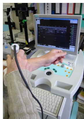
Figure 7: Photograph of the high frequency (20 – 50 MHz) ultrasound imaging system [17] (for in vivo human forearm skin images).
