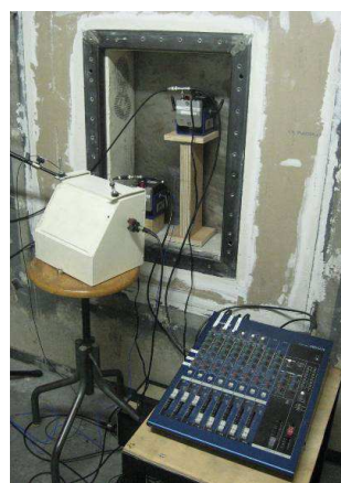
Photo 2: Excitation room (shakers, loudspeaker and table mixer)
