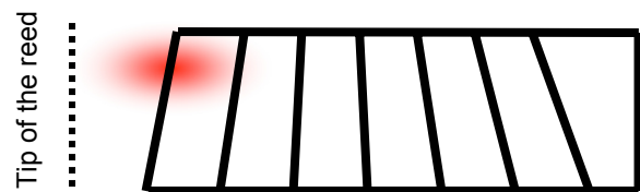
Figure 7: Top view of the Claripatch for a local reduction of the stress on the right side only. The clarinetist scrapes the reed approximately in the red area, if the playability of the reed is advantageously improved by this patch.
