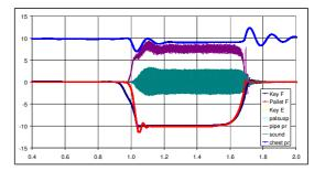
Figure 10: Effect of the variation on the pressure in the wind system due to the playing of a note. Model organ University of Edinburgh
