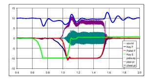
Figure 11: Effect of the variation on the pressure in the wind system due to the release of a note on a subsequent note. Model organ University of Edinburgh
