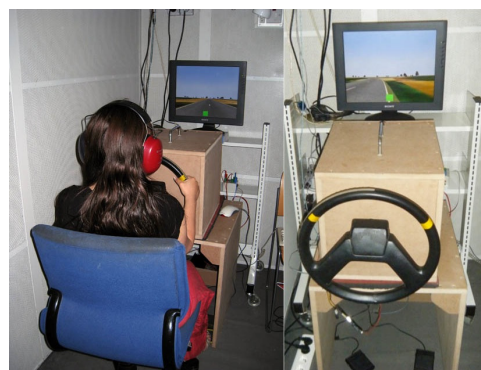
Figure 3: The test bench. The vibrating steering wheel is equipped with pressure sensors FSR. The computer screen depicts a road trajectory; a visual rectangle indicator (middle of the screen at the bottom) gives the pressure feedback on the steering wheel (green on the picture). Two pedals are used as response interface during experimental tasks.
