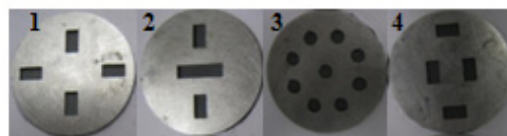
Figure 5. MPPs and MSPs with different perforations distribution.
