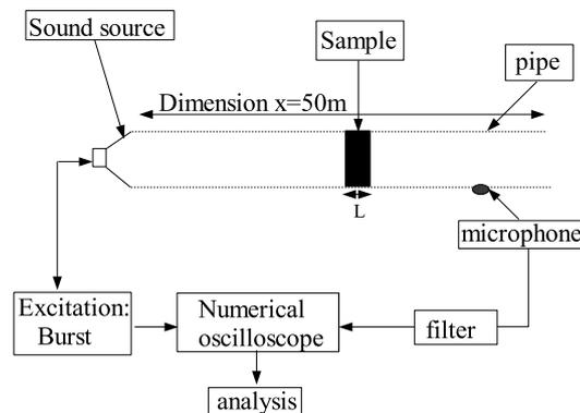
Figure 1: Experimental setup of acoustic measurements. For measuring the viscous and thermal tortuosity, porosity and thermal permeability, a length of 3m of the pipe is enough because the frequencies used in the experiment are higher than 1 kHz. The cut-off frequency of the tube is  $f_c \approx 4kHz$ . A sound source Driver unit “Brand” constituted by loudspeaker Realistic 40-9000 is used. Bursts are provided by synthesized function generator Stanford Research Systems model DS345-30MHz. The
