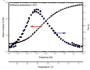
Figure 2: Reduced frequency nomogram of a standard polyvinylbutyral [9].
