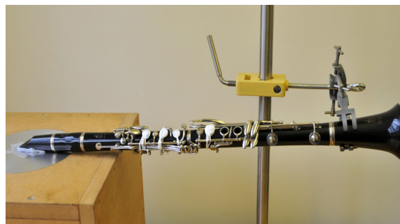
Figure 4: Buffet B12 clarinet mounted on in-house capillary-based impedance measurement system.
