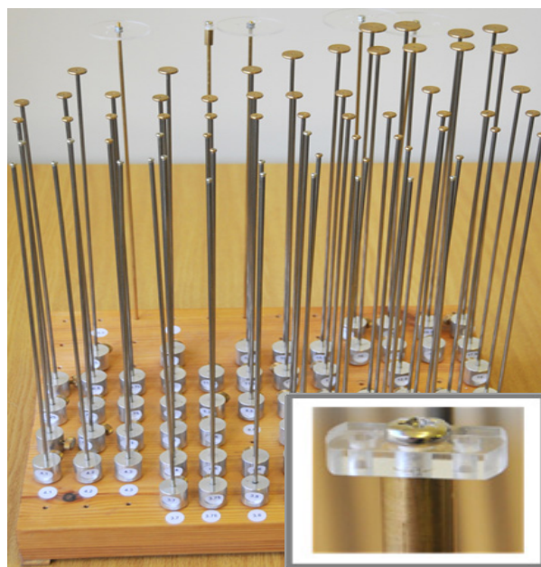
Figure 2: Set of measurement discs and rods; a cut-down disc is highlighted.
