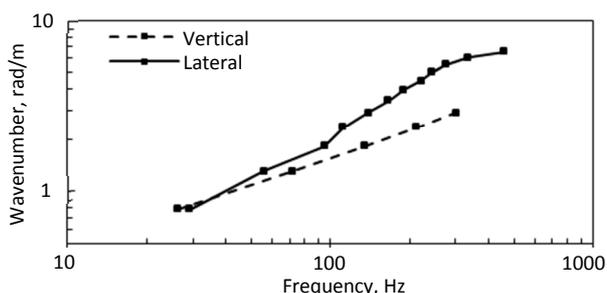
Figure 7: Dispersion curves for 6 m rail with dampers fitted.
