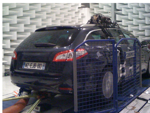
Figure 10: Peugeot 508 on a roller bench.
