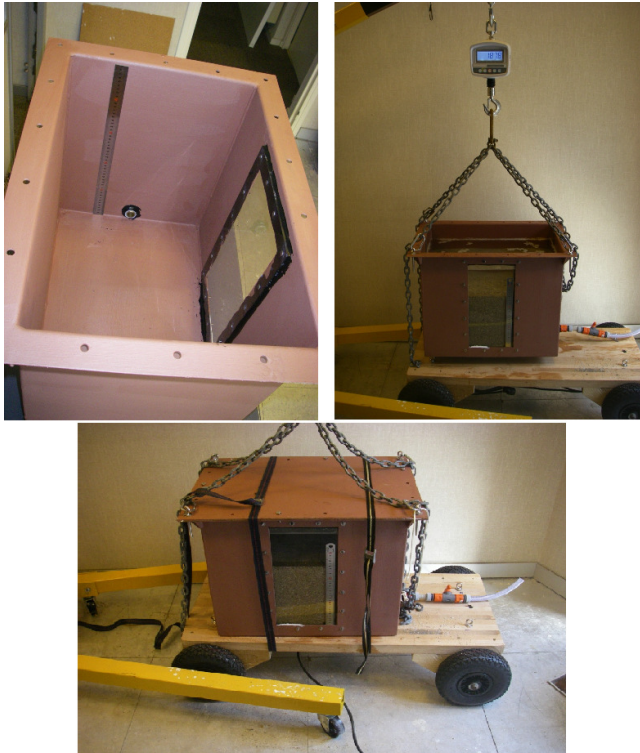
Figure 3: Top left, picture of the tank. Top right, balance for the tank filled with sediment and water. Bottom, tank on the vibrating table.
