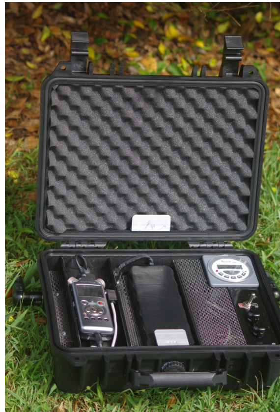
Figure 3: The recorder based on the Olympus LS-11, with large external battery, timer and AGC card all housed in a waterproof case.
